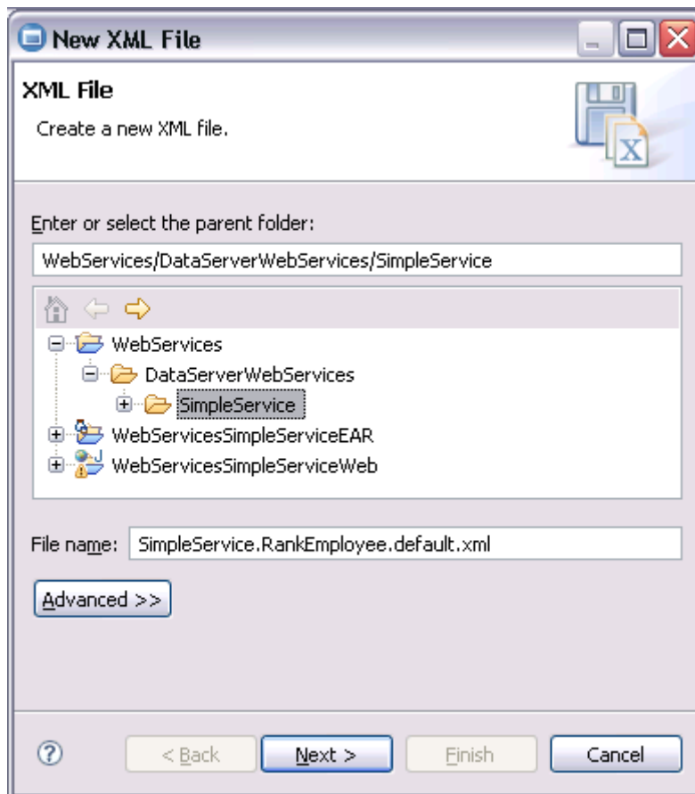
Figure E.3 – Selecting an XML file name and location
