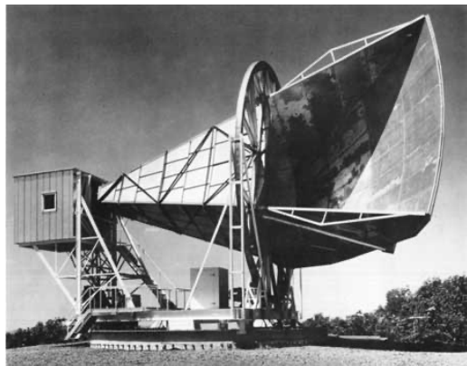
Horn antennas, Penzias and Wilson detection of the CMB radiation, proof of Big Bang
